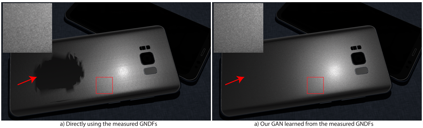
Fig. 13. The left image shows the naive approach of using the measured data for rendering directly. This is clearly not viable, and illustrates the need for some texture synthesis and hole filling in order to use this data effectively. Our GAN result learned from the measured GNDF dataset (right) shows closely matching highlight size and intensity, and similar glint appearance, but fixes the issues with holes and the visible tiling pattern.
