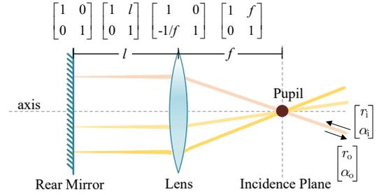
Fig. 4. Telecentric cat's eye retroreflector
