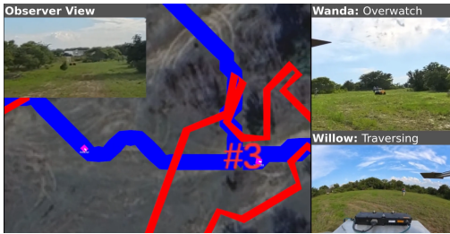
Fig. 18. Overwatch view of robot Wanda while robot Willow traverses an edge. Observer view in the top left corner shows the traversing robot being detectable from the observer perspective.
