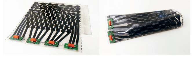
Fig. 4. Left: Our prototype sensor with connector boards. Both conductive layers contain 12 electrode strips each, and the overlaps amount to 92 sensor cells. Right: Using silicone glue, the topology of a flat sensor can be changed to form e.g. a cylinder. See Fig. 14 for our second and larger fabricated sensor.
