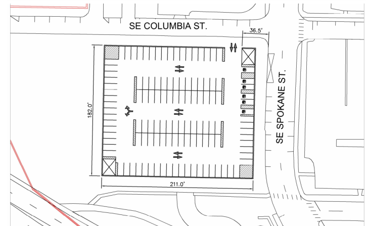
LID LEVEL PARKING LAYOUT LID SURFACE TO MATCH ELEVATION OF SPOKANE ST. (-2445'-0")
