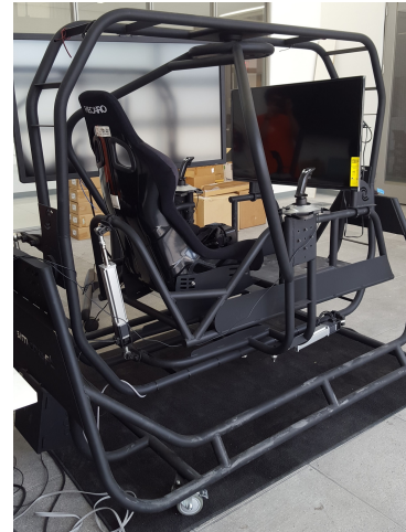
Figure 3: Motion simulator hardware with 3-axis motor actuators.
