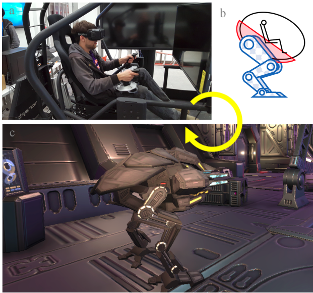
Figure 1: Conceptual layout: a) User provides input while housed in hardware full-body haptic rig. b) Physical proxy for player’s avatar, translates input to movement. c) Proxy interacts with MechVR game environment
