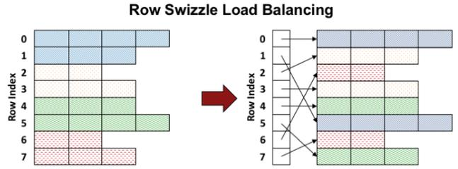
Fig. 6. **Row swizzle approach for load balancing sparse matrix computation.** Rows processed by the same warp are marked with the same pattern and color. We introduce a layer of indirection that re-orders when rows are processed. To balance work between threads in a warp, we group rows of similar length into *bundles*. To balance work between SMs, we process row bundles in decreasing order of size.
