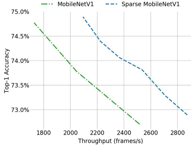
Fig. 12. **MobileNetV1 accuracy-runtime tradeoff curves.** Sparse modes are more efficient, achieving speedups of 21-24% for a given accuracy across all model sizes, or equivalently, ~1.1% higher accuracy for the same throughput.
