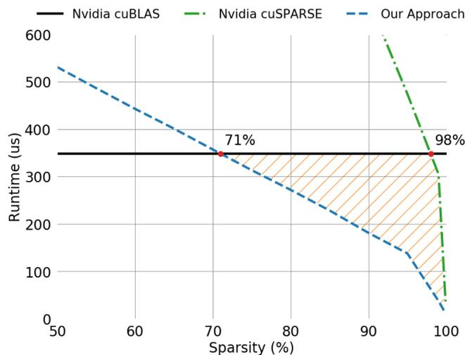
Fig. 1. **Sparse matrix–matrix multiplication runtime for a weight-sparse long short-term memory network problem.** Input size 8192, hidden size 2048, and batch size 128 in single-precision on an Nvidia V100 GPU with CUDA 10.1. Using our approach, sparse computation exceeds the performance of dense at as low as 71% sparsity. Existing vendor libraries require 14 $\times$  fewer non-zeros to achieve the same performance. This work enables speedups for all problems in the highlighted region.
