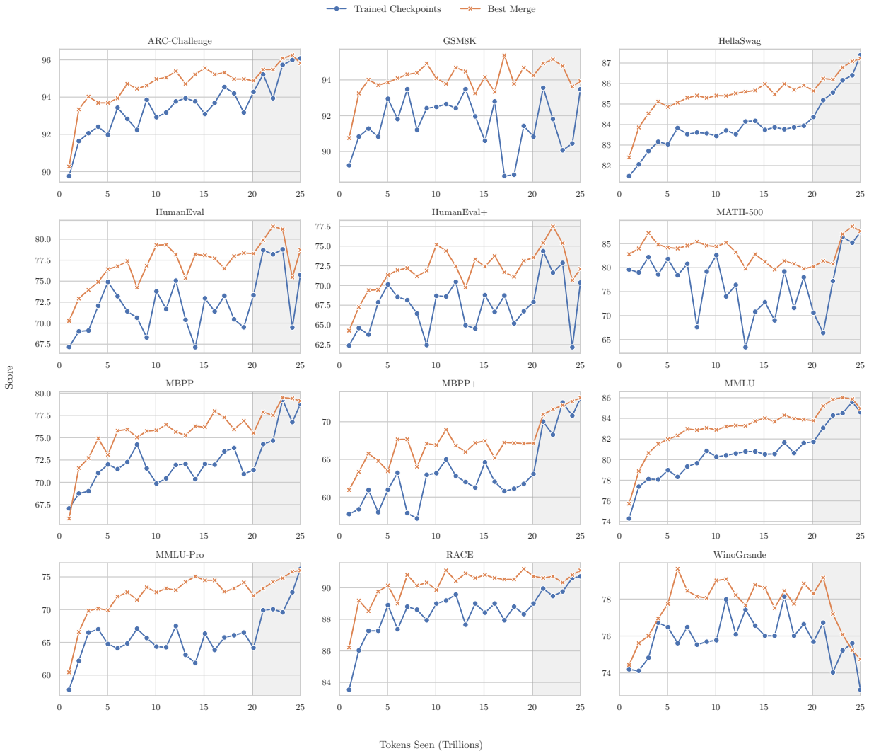
Figure 17 | Per-benchmark accuracy for trained checkpoints versus the best offline checkpoint merge across the full 25T-token training run. The 12 benchmarks span general knowledge (MMLU-Pro, MMLU), code generation (HumanEval, HumanEval+, MBPP, MBPP+), mathematical reasoning (GSM8K, MATH-500), and commonsense understanding (RACE, ARC-Challenge, HellaSwag, WinoGrande). The shaded region indicates the LR decay phase.
