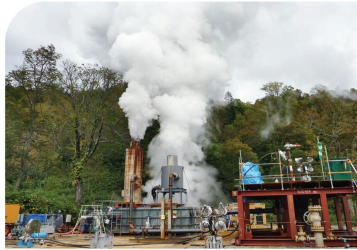
Steam emerges from a well dug to test geothermal power generation in Hokkaido in October 2015. | KYODO
